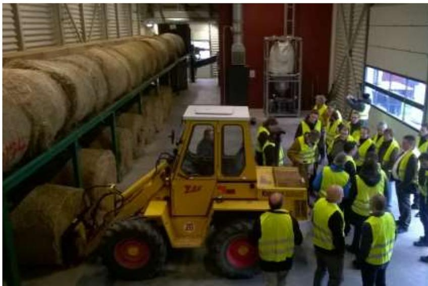
Fig.: Automatic fuel supply at the heating plant 980 kW in Ringsheim, Southern Germany. Bales are made from hay harvested on mountain grass meadows nearby. In future there should be plenty of these plants in place for utilisation of biomass from rewetted peatlands.
